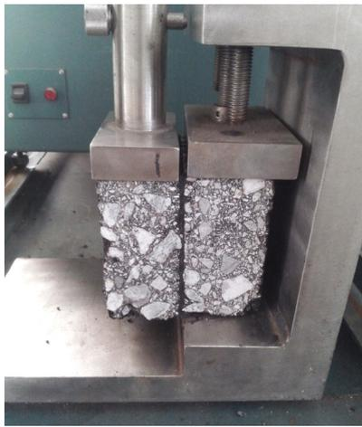
Fig. 1. Shear bond strength test
